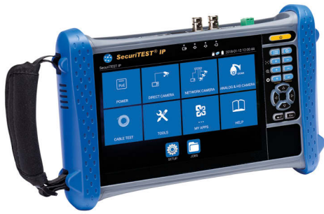
CCTV Camera Tester for IP Digital / HD Coax / Analog Systems
