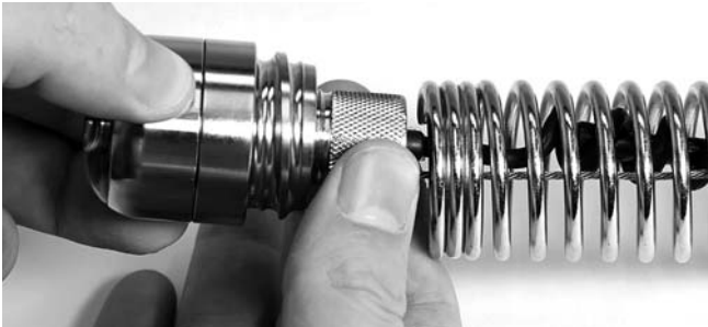
Figure 36 – Removing Camera Head From Locking Sleeve
