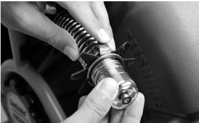
Figure 14 – Pre-stressing The Flanges
