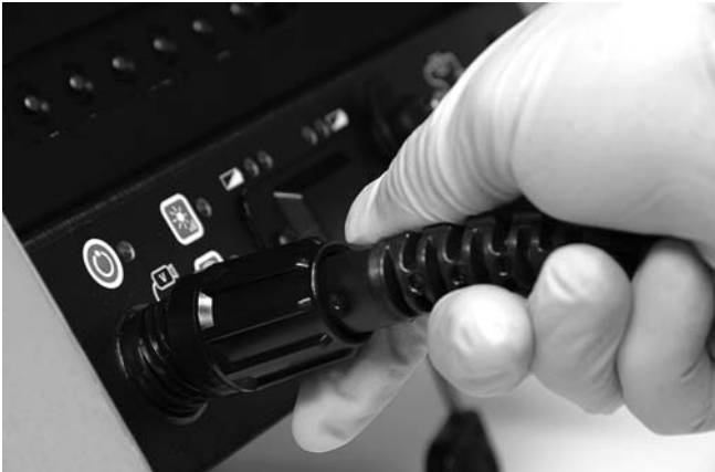
Figure 17 – Connecting To A SeeSnake CCU
