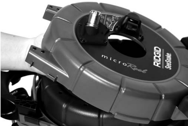
Figure 5 – Open Drum Carefully To Route Cable
