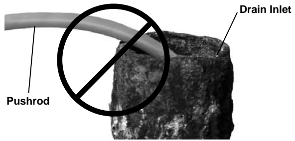
Figure 23 – Avoid Pulling At Sharp Angles
