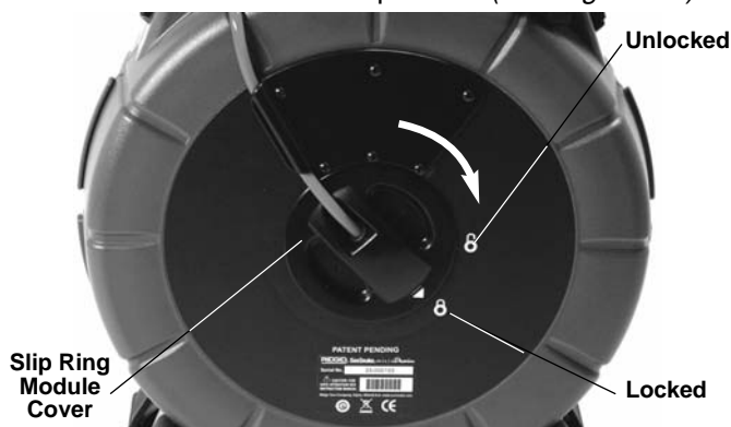
Figure 11 – Locking The Slip Ring Module Cover
