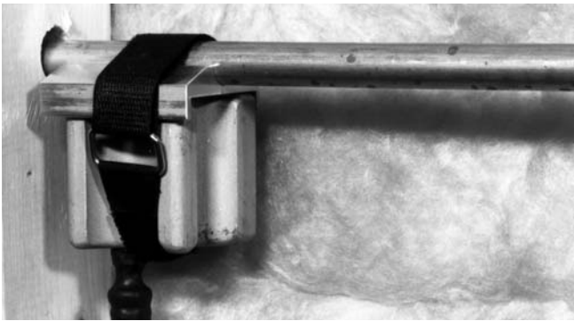
Figure 7 – Freeze Head with End Adapter Attached with Velcro Strap
