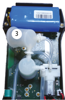
Sensor removed from white rubber cap
