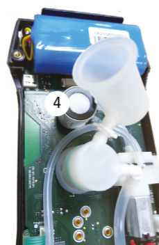
New sensor connected to electronic board
