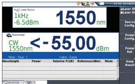
Built-in power meter and laser source
