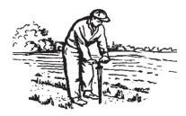
Using a soil auger, soil sampler, or posthole digger, you can insert Delmhorst Gypsum Blocks at any depth to best suit the root structure of each crop, since moisture is checked in areas of active root growth.
