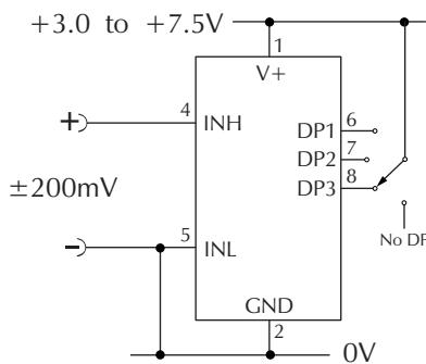
Measuring a single ended input voltage referenced to supply, i.e. the input voltage and the meter's power supply share the same 0V rail.
