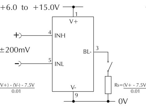
Measuring an input voltage referenced to a floating supply, i.e. the input voltage and the meter's power supply are isolated from each other.
