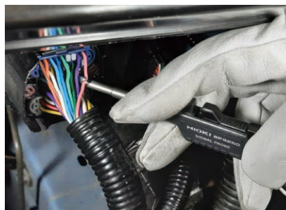
Quickly pinch with one hand from over the sheath
