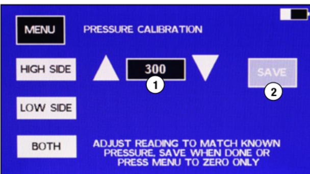
**Note:** Do not press SAVE if the pressure in the manifold does not match the pressure displayed. To exit without saving, press MENU.
