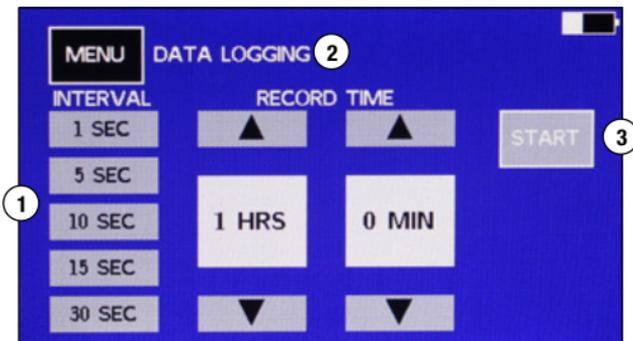
1. Press on the interval that the data samples will be recorded to highlight it.
