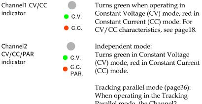
When operating in the Tracking Parallel mode, the Channel2 indicator always stays red (PAR). Channel1 indicator shows the CV/CC status.
