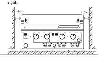
Cooling fanThe cooling fan is located on the rear panel.openingAllocate extra space on the back of SPD-3606 so<br/>that the cooling fan opening would not become<br/>blocked.
