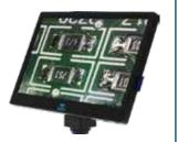
By attaching an inspection camera onto the port of your trinocular microscope, you can view your inspection on a monitor and digitally save images. USB models connect to your computer and require software for image capture, measurement and annotation. HDMI cameras connect directly to an HD monitor and save images to a SD card or USB flash drive. Advanced HDMI cameras have integrated imaging/measurement software.
