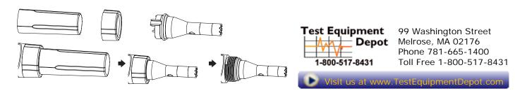
The membrane part is replaceable.
