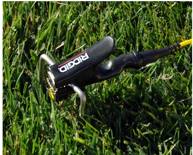
Figure 5 – Connecting the ST-305 Ground Stake
