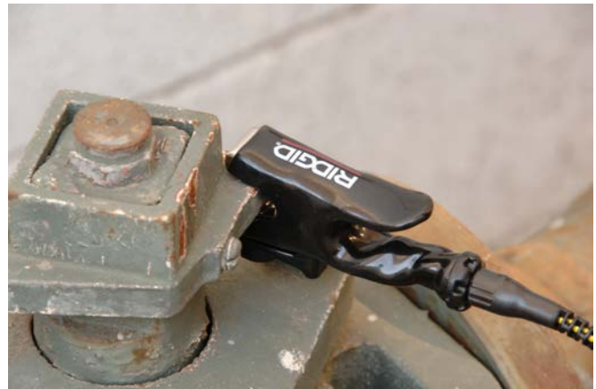
Figure 6 – Connecting the ST-305 using the clip
