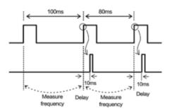
If the period of the external input is less than the setting of the delay time, the delay time is ignored and the ST-329BL flashes as if the delayed time equals 0.
