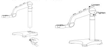
After adjusting the tension knob to some extent, the upper arm can be move up and down. When the pH electrode is placed on the arm and calibration or measurement is being performed, the storage bottle of pH electrode can be placed into the base hole for easy storage:
