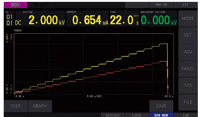
Example of stepped voltage rise testing
