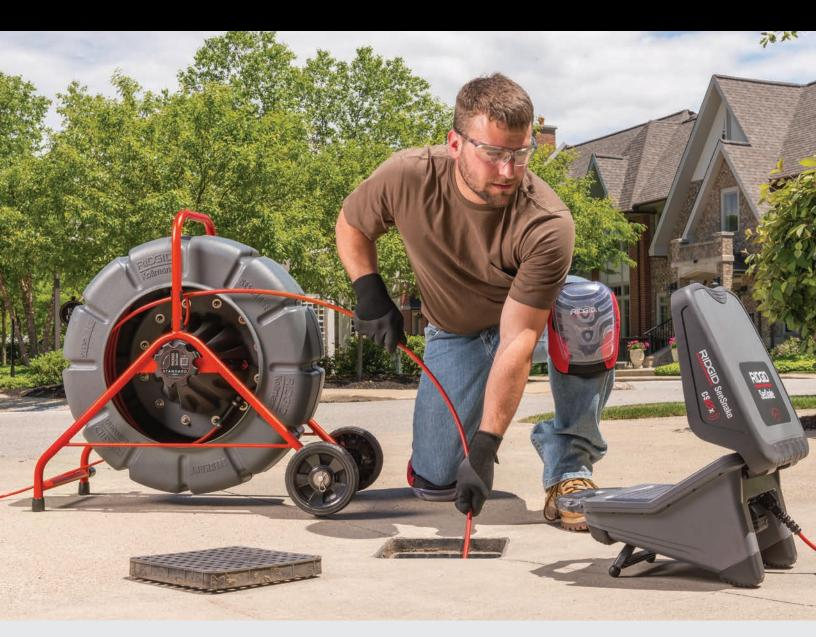
Equipped with the largest diameter SeeSnake® camera head, the Standard is your go-to machine for inspecting long runs in main sewer laterals. Everything about the Standard suggests durability, from the all-metal frame and hardened stainless steel camera head to the stiff cable. Newly available TruSense technology provides a high dynamic range (HDR) image sensor and a TiltSense™ inclinometer for SeeSnake CSx series Wi-Fi enabled monitors.
