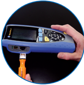
No calibration required plus replaceable RJ45 contacts
