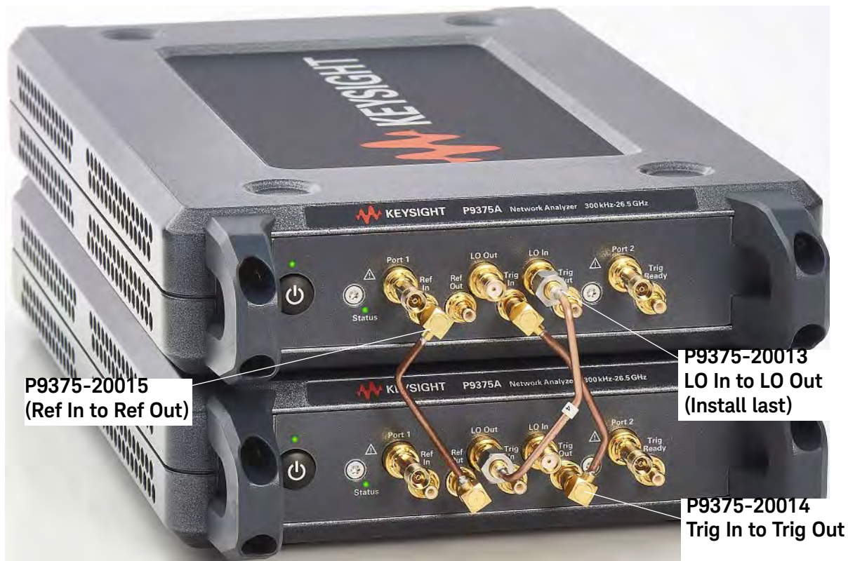
Figure 1-8 Installing Semi-Rigid Cables from Option Y1701A—P9375-20013, P9375-20014, and P9375-20015
