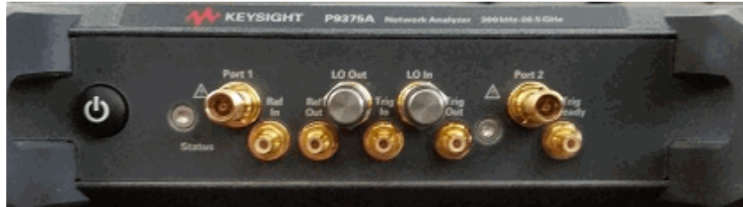
Figure 1-4 50 Ohm Loads Installed on the Network Analyzer Modules
