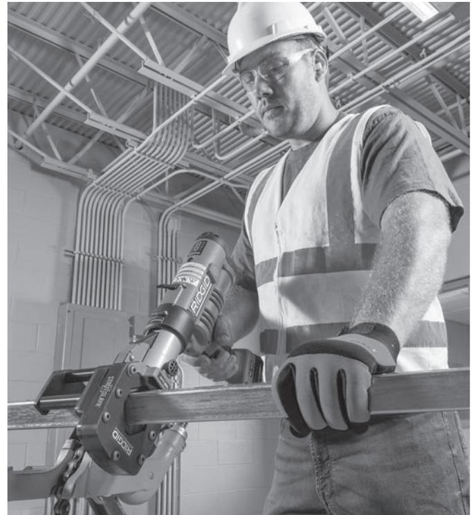
**Figure 8 – Shear In Use**
