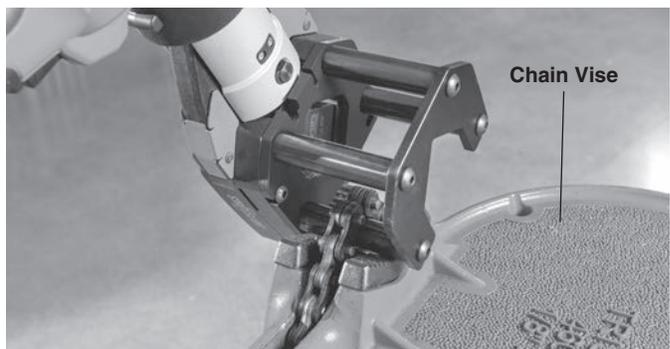
**Figure 5 – Strut Shear Head Mounted in Chain Vise**
