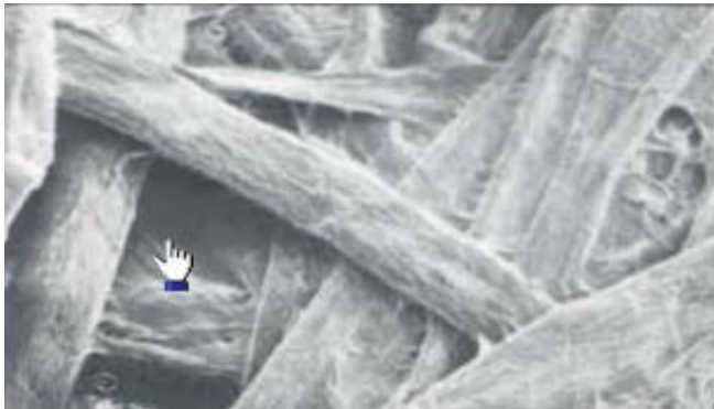
Photomicrograph of the fiber weave of a conventional filter bag (500x)
