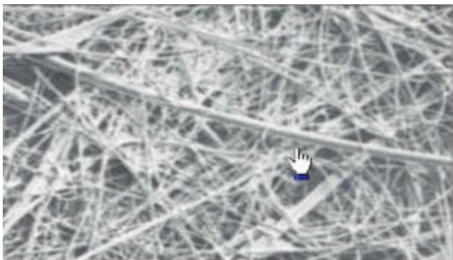
Photomicrograph of the fiber weave of a filter (500x)
