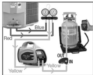
4. Connect equipment per **DIAGRAM B (RECOVER)** but **DO NOT PLACE TANK ON SCALE AT THIS TIME**
