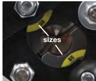
2. Select sizes on underside of dies to match tubing O.D.
