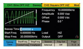
Sweep mode supports 'Linear' and 'Log' sweep, with 'Up' and 'Down' direction, and Sweep source can be configured as 'Internal', 'External' or 'Manual'.
