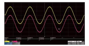
Output amplitude into a high impedance load can be as high 20 Vpp at frequencies up to 20 MHz, and 10 Vpp for frequencies greater than 20 MHz.
