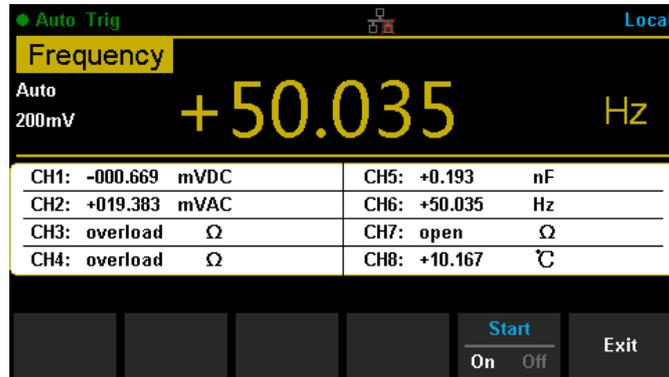
The upper part of the interface displays the function, range, and result of the current channel. The table below records the measurement result of each channel.
