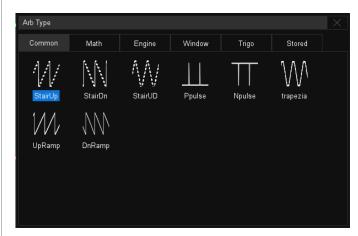
The built-in waveform generator can output waveforms with up to 25 MHz frequency and ±3 V amplitude. Six basic waveforms together with multiple types of predefined waveforms and as user-defined arbitrary waveforms are supported.
