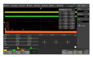
T3DSO3204: At 200 MHz bandwidth, the input noise floor is typically only 80  $\mu$ Vrms.
