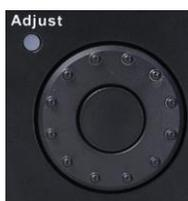
During menu operation, when the light in the upper left corner of the knob is on, you can turn the knob to select among the submenus under the current menu, and press down to select the current submenu. Additionally, it can also be used to modify parameters and input filenames.
