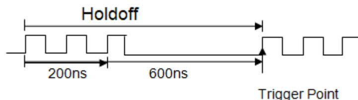
The correct holdoff setting is typically slightly less than one repetition of the waveform. Set the holdoff to this time to generate a unique trigger point for a repetitive waveform. Only edge trigger and serial trigger have holdoff option. The holdoff time of the oscilloscope is adjustable from 80ns to 1.5s.
