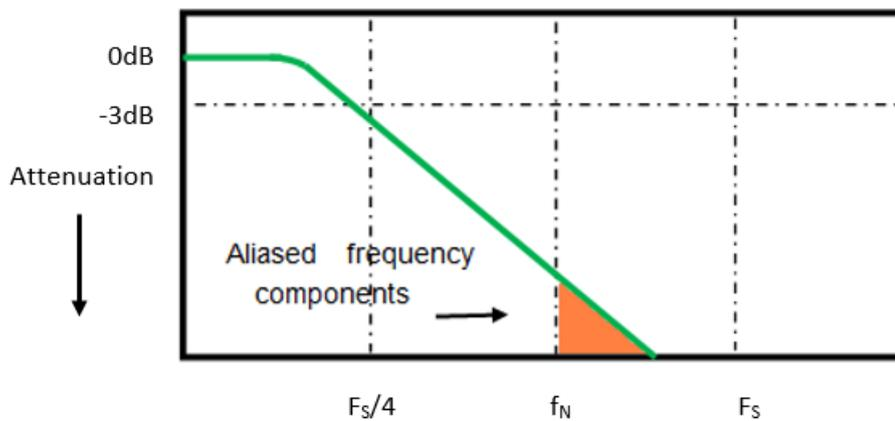
Limiting oscilloscope bandwidth ( $f_{BW}$ ) to  $\frac{1}{4}$  the sample rate ( $f_s/4$ ) reduces frequency components above the Nyquist frequency ( $f_N$ ).
