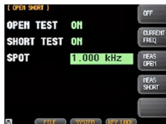
Selectable Fixture Zeroing Methods Full Frequency Range Zero or Spot Frequency Zero
