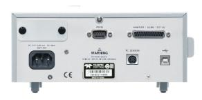
T3MIL series provides a D-sub 25-pin combined interface to control the device for various functionalities such as Handler, Scan and EXT I/O. Handler function can be used for connecting the device to a sorting machine in a production environment. Scan and EXT I/O is useful when connecting to an external switch or for an external trigger control. T3MIL series also offers remote control and data retrieval through various interfaces such as RS 232C and USB.
