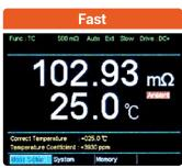
T3MIL series offers Fast (60 readings per second) and Slow (10 readings per second) measurement speeds.
