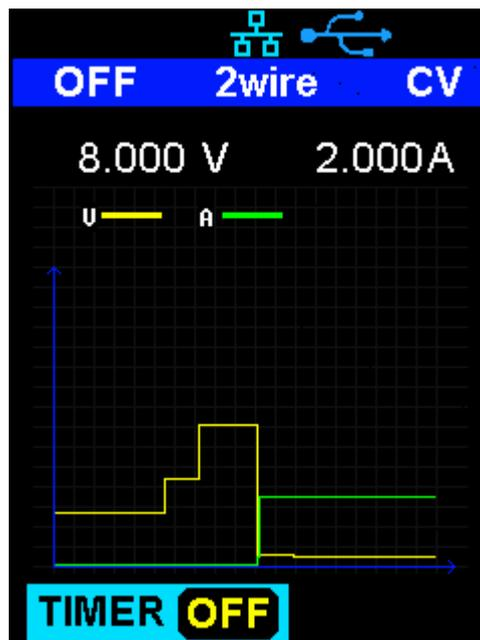
**Note:** The yellow line indicates the voltage output curve, the green line indicates the current output curve, and the ordinate axis indicates the output value.
