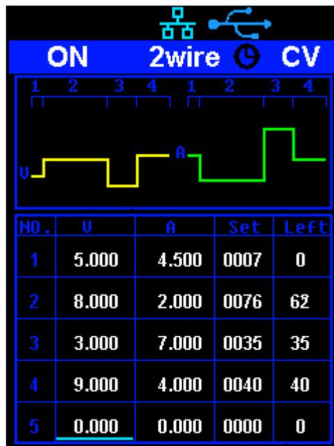
After starting the timer function, the timer will stop if you press the **On/Off** button to switch off the channel output. When the channel output is turned on again, the timer will continue counting from the last point in time it stopped. After the countdown steps have completed the timer will turn off automatically.
