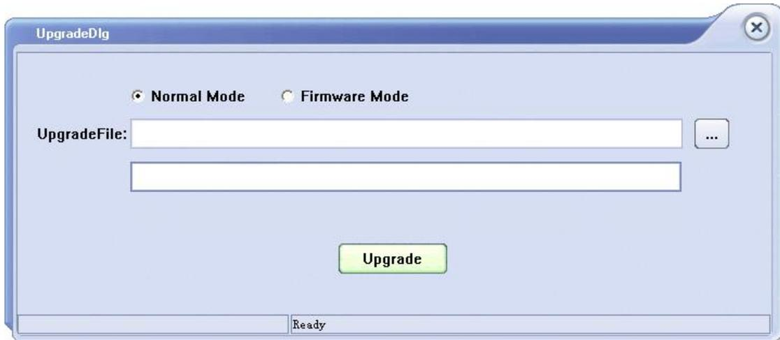
4. Click the Upgrade button to begin the upgrade. The upgrade is finished when the progress bar completes and the instrument will automatically run the version after the upgrade.
