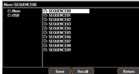
3. Rotate the scroll wheel (Encode) to select target file.
