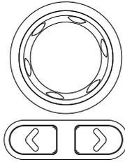
Scroll wheel is used to set each parameter value, whilst arrow keys are used for parameter, menu selection and voltage/current fine adjustment. It is used to switch or operate the displayed waveforms under diagram display mode.
