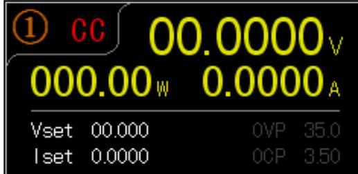
**Description** Each channel is equipped with basic power functions and able to display both settings and read back value of V/I as well as output status
