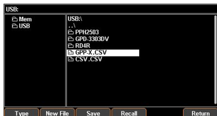
5. Press F3 (Save) button to save the settings of Sequence into the corresponding file.
