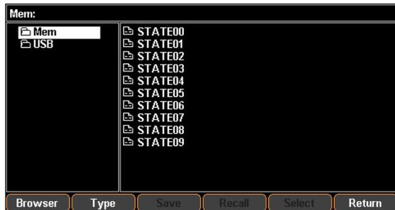
2. Press the right arrow button to enter the file group. Rotate the scroll wheel (Encode) and stop at the file in need
