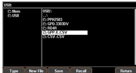
5. Press F3 (Save) button to save the settings of Delay into the corresponding file.
