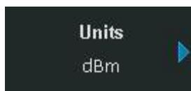
Press the corresponding menu key to enter the lower menu and change the option currently selected. For example, press **Units** to enter the lower menu. Select **dBm** and return to the previous menu. The unit of Y- axis changes to dBm.
