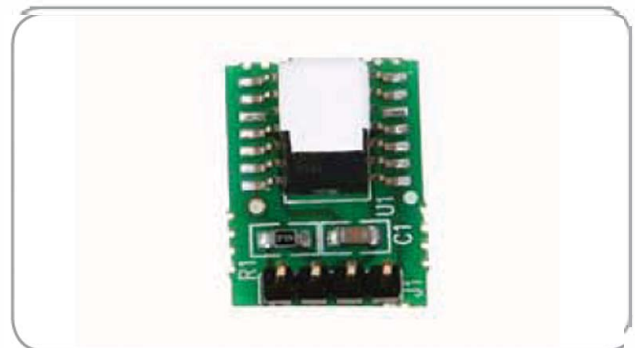
Replaceable, humidity sensor. Specially designed hydrophobic filter to prolong sensor calibration life.
