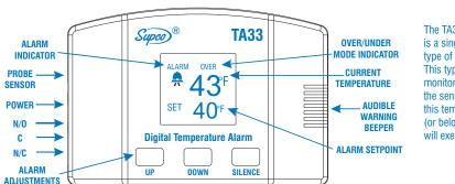
The TA33 Temperature Alarm is a single point or threshold type of temperature alarm. This type of temperature alarm monitors the temperature at the sensor probe tip and when this temperature passes above (or below) the set point, the unit will execute a preset operation.
