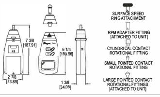
The MODEL TAC-L Portable Digital Tachometer measures rotational speed either by contacting a rotatable head to he shaft of the object or by using a photo sensor to detect the reflections from the laser. The housing is made of a strong, lightweight ABS plastic housing, which is designed to comfortably fit in the hand of the user. Supplied with this model are 3 contact rotational heads, a contact surface wheel, and a protective carrying case.
