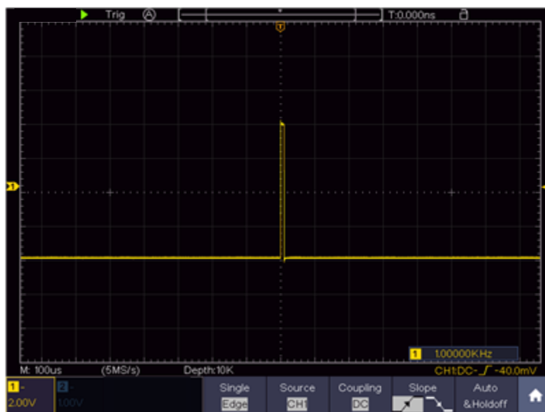
Figure 8-3 Capturing a Single Signal
