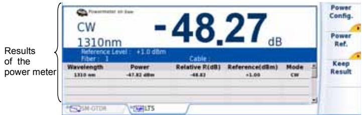
Fig. 14 Results and commands of the power meter
