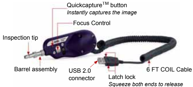
Fig. 16 P5000 Probe components
