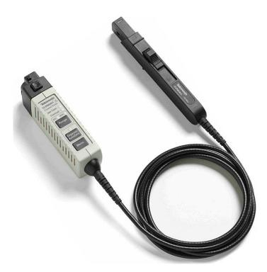
TCP0030A is a high-performance, easy-to-use AC/DC current probe designed for use and direct connection to oscilloscopes with the TekVPI<sup>™</sup> probe interface. This AC/DC current measurement probe provides greater than 120 MHz of bandwidth with selectable 5 A and 30 A measurement ranges. It also provides exceptional low-current measurement capability and accuracy to current levels as low as 1 mA, important for meeting today's challenging current measurement needs.
