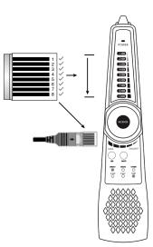
by sound: the "di" sound means connected pair lines, while the "du" sound means short circuit pair lines. All indicator lights of short circuit pairs are on at the same time.
