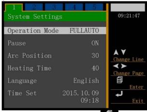
Press the keys "▲", "▼" to move the cursor; press the key to enter the program that you want to get into; press again the keys "▲" to modify the parameter values (via moving the cursor)
