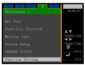
Press "▲" "▼" to move the cursor, press to enter the program that you desire to get into, press "▲" "▼" over again to modify the parameter values(via moving the cursor in the small pane);
