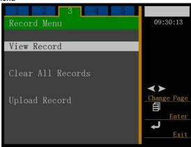
Press to enter "View Record" Menu, and press "◄", "▶" to select and view the Fusion-Splicing Records.
