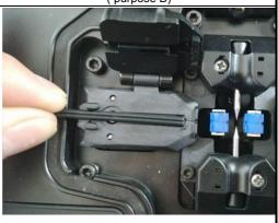
2. Steps of Assembling and removing "removable guiding groove": Holding the tail of "removable guiding groove", lift it up and forward, and take out. As below pictures:
