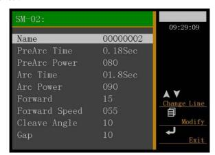
Press "▲" "▼" to move the cursor; press to enter the menu which needs to be modified; press "▲" "▼" to modify the parameters; Press over again to confirm and save it. After completing the modification, press to exit.
