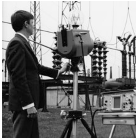
1969: Thermovision Model 661. The camera weighed approximately 25 kg (55 lb.), the oscilloscope 20 kg (44 lb.), and the tripod 15 kg (33 lb.). The operator also needed a 220 VAC generator set, and a 10 L (2.6 US gallon) jar with liquid nitrogen. To the left of the oscilloscope the Polaroid attachment (6 kg (13 lb.)) can be seen.
