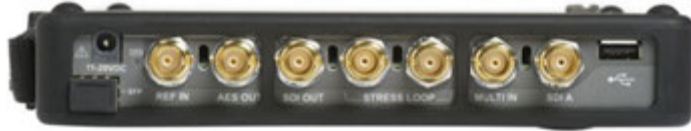
WFM2300 top panel connectors.
