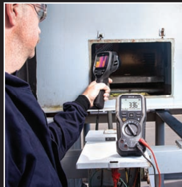
METERLiNK connectivity to FLIR IR cameras
