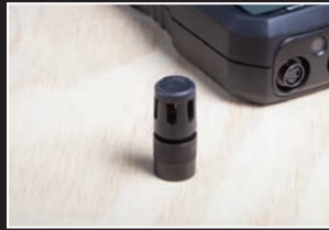
Temperature/humidity sensor is field replaceable
