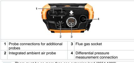
There must be no more than one extension lead (0554 1202) connected between flue gas socket and flue gas probe.
