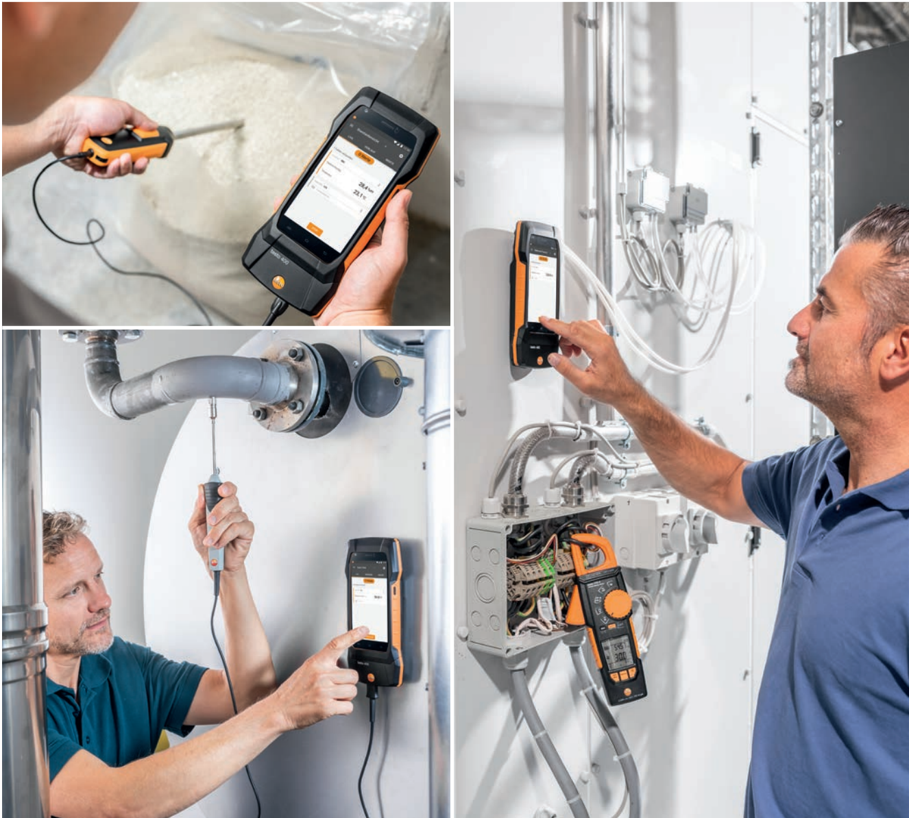
With the testo 400, you can use up to eight probes simultaneously (4 x Bluetooth, 4 x cable).
