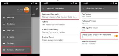
If a new firmware is available for your measurement instrument, an update notification is shown after connecting the instrument with the testo Smart App.
