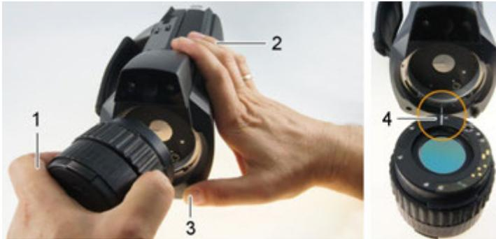
1. Grip the lens with your left hand (1), hold the imager with your right (2) and press **[Release lens]** (3).
