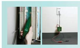
Non-Contact probe audibly identifies selected wire or cable. Easily trace wires from source to termination.
